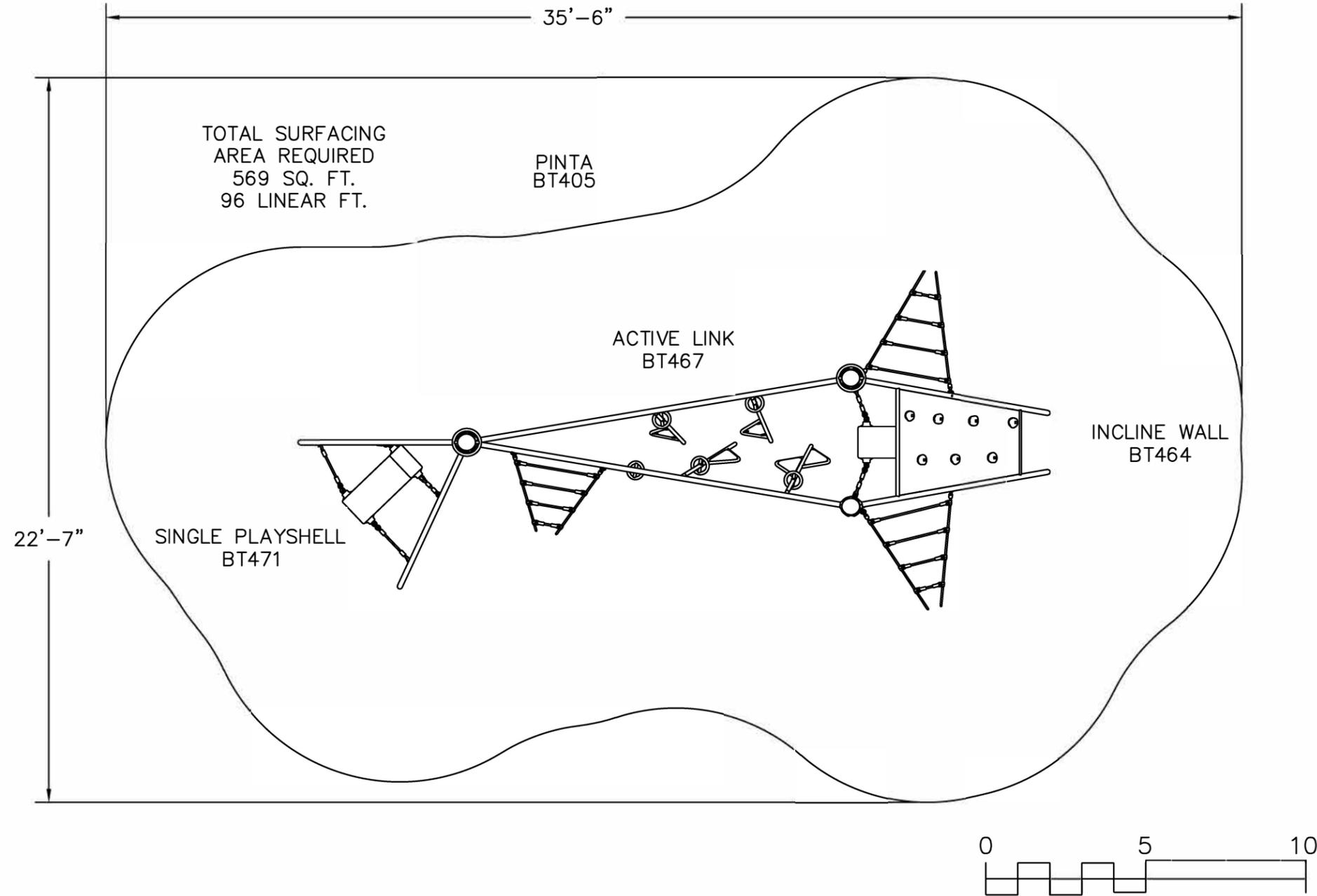
**IMPORTANT:** Never install play equipment over hard, unresilient surfaces such as asphalt, concrete, or compacted earth. It is the owner's responsibility to ensure the "minimum area required" contains an appropriate amount of resilient material to cushion accidental falls.
