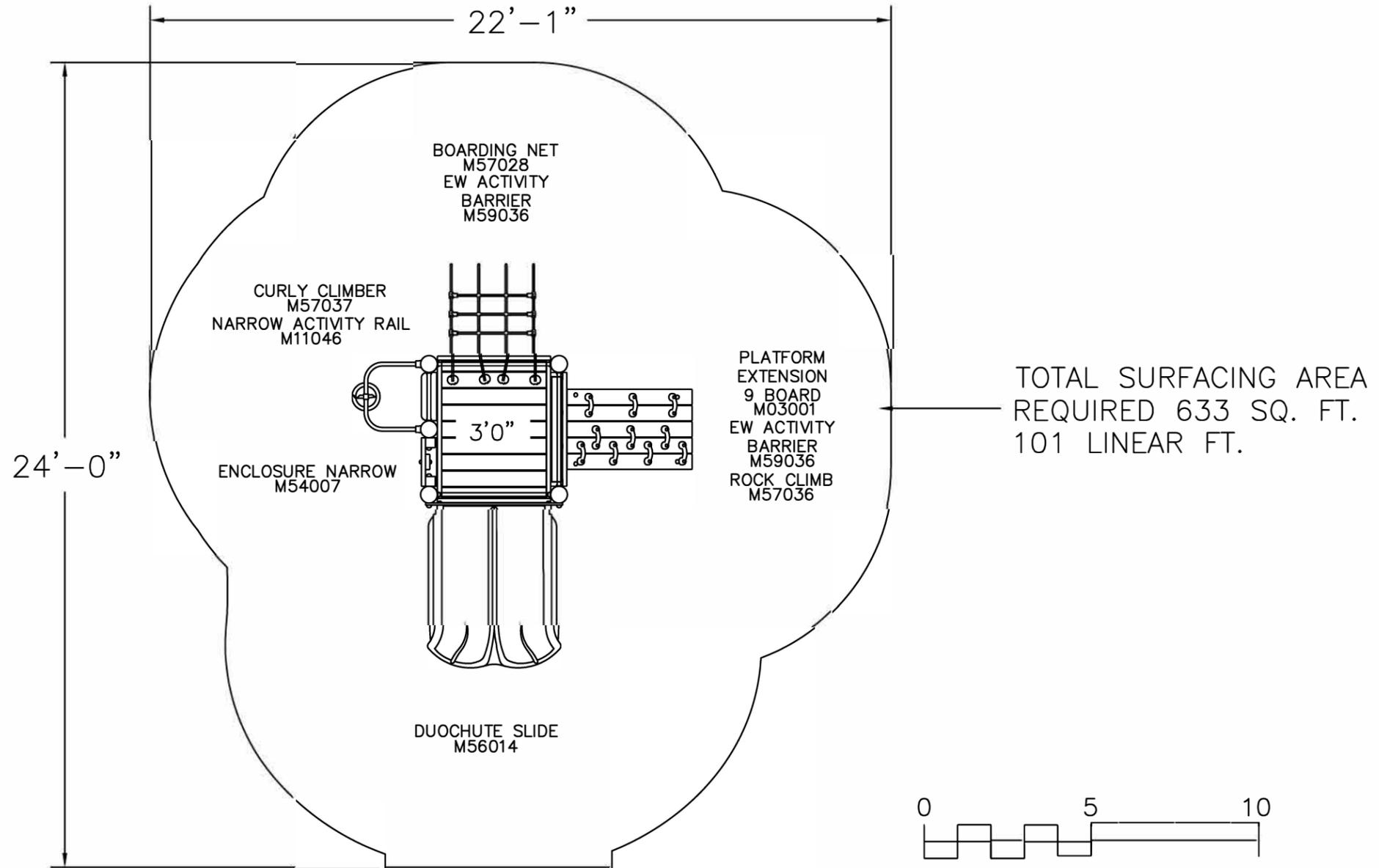
**IMPORTANT:** Never install play equipment over hard, unresilient surfaces such as asphalt, concrete, or compacted earth. It is the owner's responsibility to ensure the "minimum area required" contains an appropriate amount of resilient material to cushion accidental falls.
