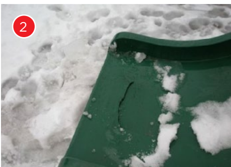
This tear could be an entanglement hazard.
