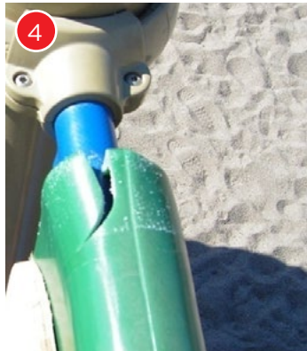
This cracked component is a hazard.
