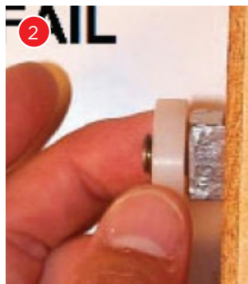
This bolt end is an unsafe protrusion.
